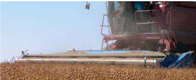
TOP / Straight-cutting allows the operator to adjust stubble height.
