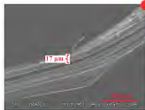
Enzyme treated fibres, separated from bundles; more single fibres. Diameter : 6 - 20 μm.
